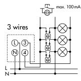
Switching with Indoor 180-SC 4-wires
