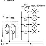
Also suitable for connection to the **B.E.G. LUXOMAT®** Indoor 180-SC. Possible expansion of detection area with a maximum of 10 detectors.
