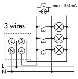
Switching with push button 4-wires
