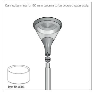
SKY can be mounted on different pole types under the condition that the top pipe is  $\emptyset 60 \times 1100 \, \text{mm}$ .
