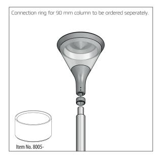
SKY can be mounted on different post types under the condition that the top pipe is  $\emptyset 60 \times 1100 \, \text{mm}$ .
