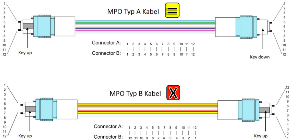
MPO Type A and MPO Type B Cables
