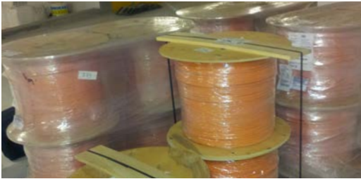
Copper cable stored in good conditions
