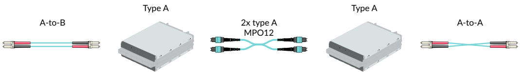
MPO polarity method A components
