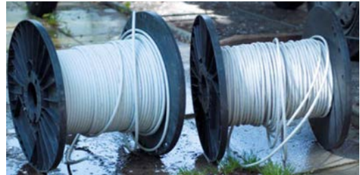
Copper cable stored in the wrong conditions
