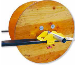
Unloading reel with bar
