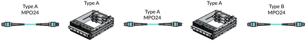
MPO polarity method A 40/100G
