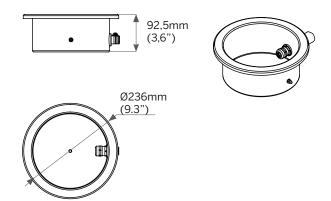
Installation housing - AL370LN \*fits 2m (6.6') cable Liner Pool Installation
