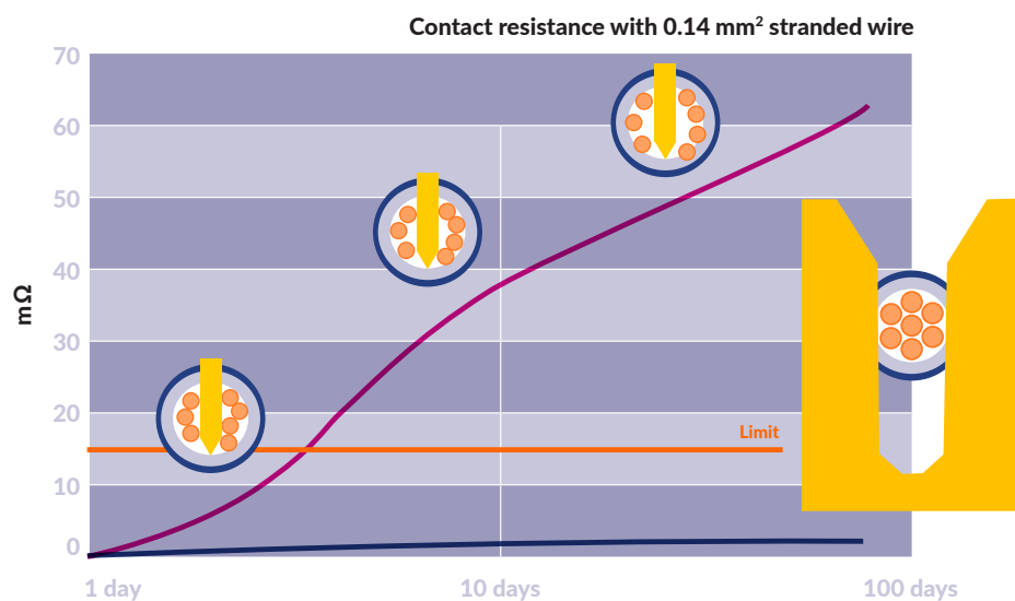
Figure 3: Resistance behavior of the piercing (IPC) and displacement (IDC) connection. IPC, violet curve: The contact resistance increases continuously, no stabilization. IDC, blue curve: The contact resistance increases just slightly and then stabilizes. Graphic: R&M
