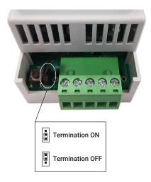
**IMPORTANT NOTE:** Connecting a mains potential cable to the iCAN Network terminals is likley to damage the unit and other devices connected, and invalidate warranty.
