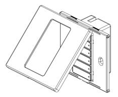
2. Unclip the face plate from the back plate.
